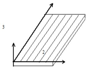
Figure 1: Lamina Reference Axes
