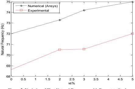
Figure 5: Variation of First Natural Frequency with Respect to Steel Volume Fraction for Hybrid Composite Plates
