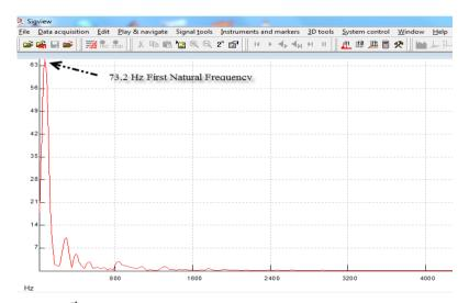
Figure 4b: 1<sup>st</sup> Natural Frequency Obtained by Experimental Test for Hybrid Laminated Composite Plate of v\_s =2%
