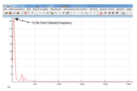
Figure 4a: 1<sup>st</sup> Natural Frequency Obtained by Experimental Test for Hybrid Laminated Composite Plate of v\_s =0%
