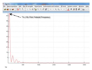
Figure 4c: 1<sup>st</sup> Natural Frequency Obtained by Experimental Test for Hybrid Laminated Composite Plate of v\_s =3%
